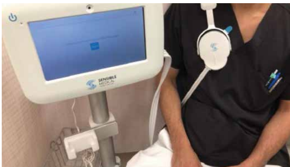
Fig. 2. Remote dielectric sensing (ReDS) technology. The device consists of two sensors (front and rear), a computing unit, and a monitor
